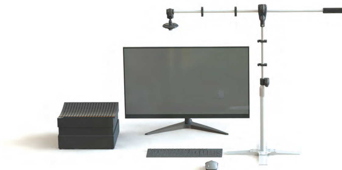
Composition of the system of the primary assessment of birthmarks “Rodinka”: process calculator, monitor for reproduction of information, camera with a bracket for image capture
