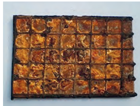
Sample after induction surfacing before machining
