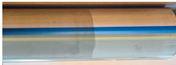
Section of the plunger subjected to magnetic abrasive processing
