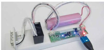
Ozonator battery charging and simultaneous ozone generation mode
