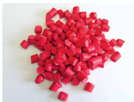
Crushed waste from EVA sprue system
