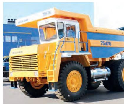
**NATURAL GAS-POWERED MINING DUMP TRUCK**
