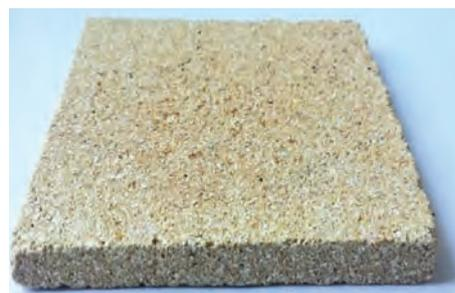
Thermostable and heat-insulating composite materials
