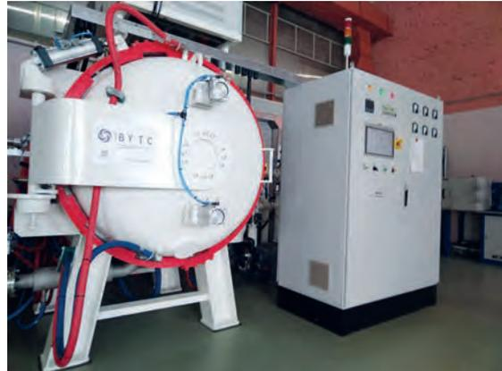
Wafer sintering equipment
