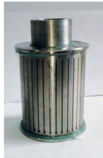
Model for hydro and (or) pneumatic testing
