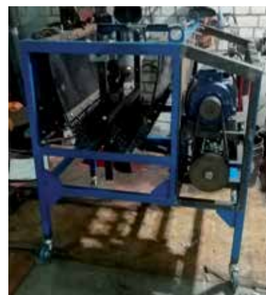
General view of a screen-disperser with a two-wave working surface based on a chain cloth
