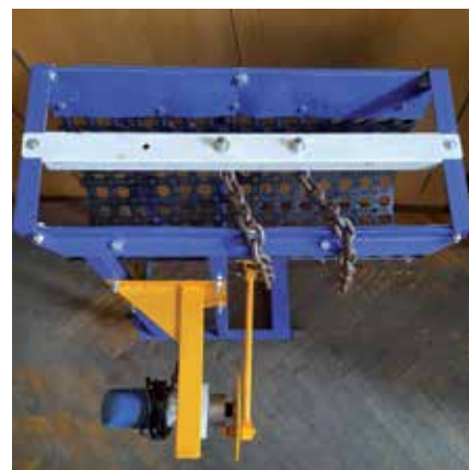
General view of a screen with a flexible single-wave screening surface
