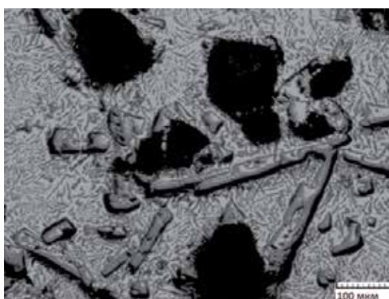
Results of optical metallographic analysis of composites with up to 15 % alumina phase
