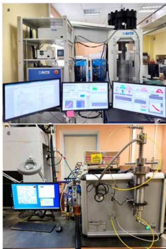
a) GCTS RTR-4500 Rock Testing System b) Instrument for Rock Filtration Properties measuring Kortekh SMP-PP
