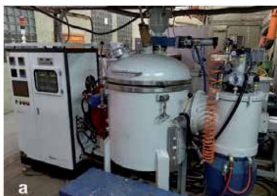
Melting equipment: a — vacuum induction furnace; b — Muffle electric resistance furnace
