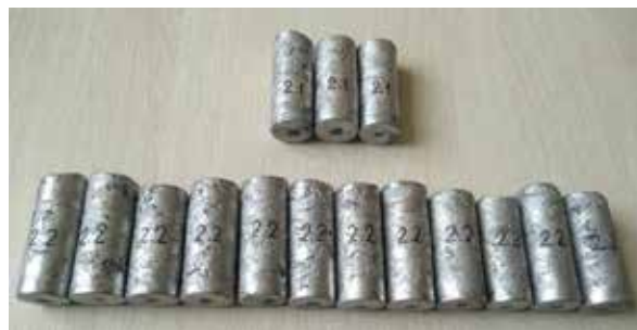
Samples of composite alloys produced using coarse silica sand from a liquid-solid-phase composition
