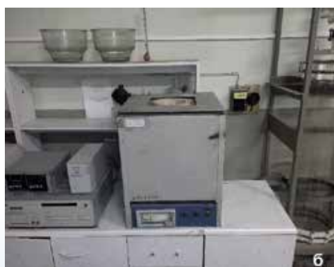
Melting equipment: a — vacuum induction furnace; b — Muffle electric resistance furnace
