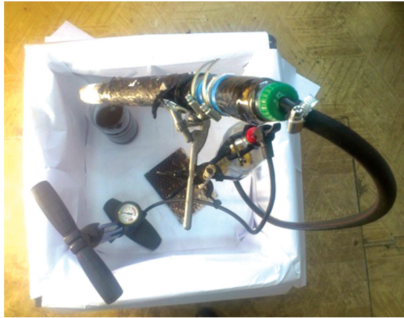
Installation for pressurizing the oil in the cable using a handpump
