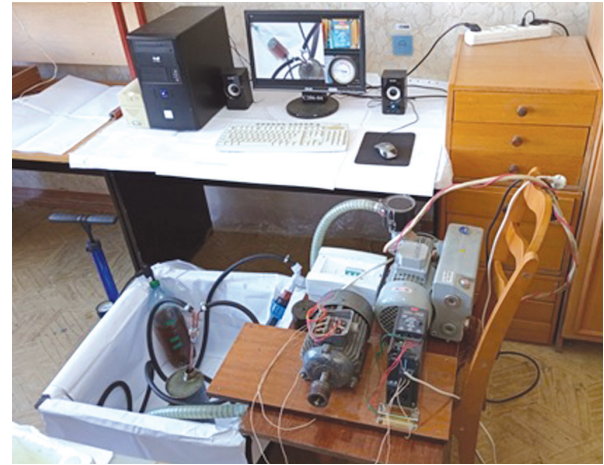
Experimental setup with a combination of hand and vacuum pumps
