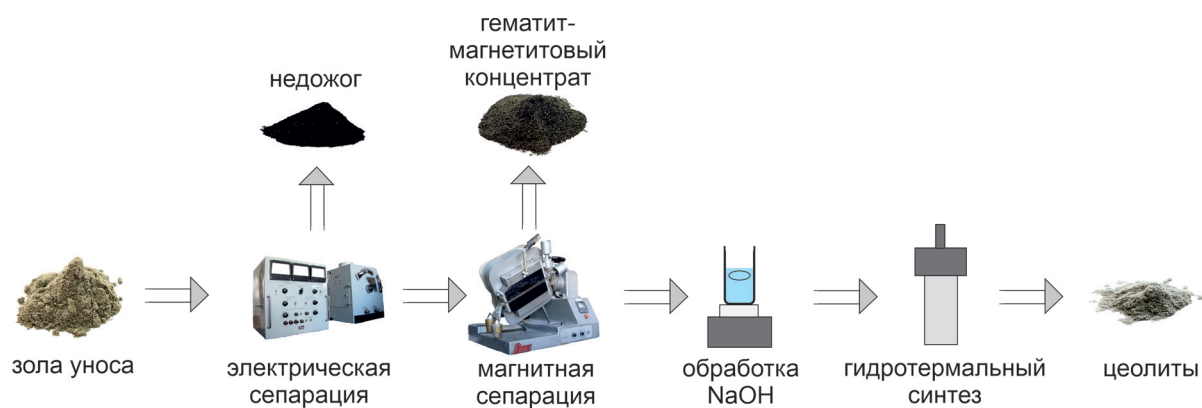
Scheme of fly ash processing
